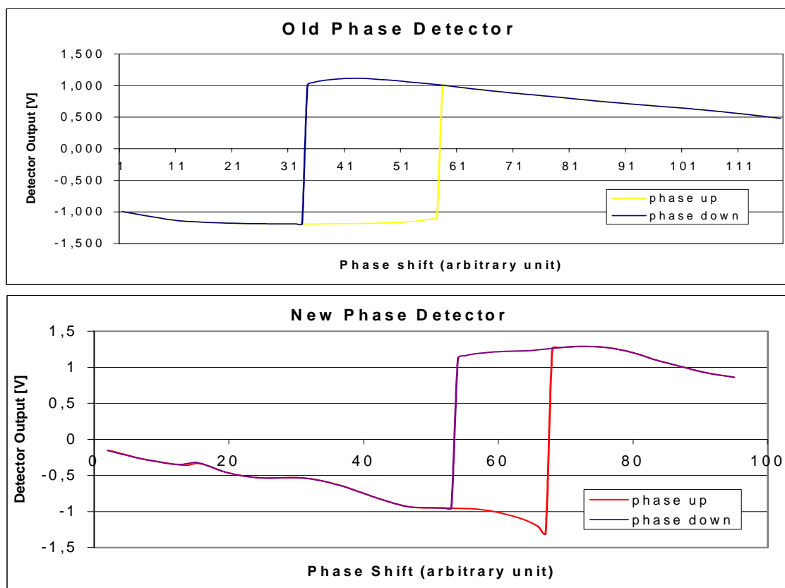
Figure 8.3.7: Hysteresis measurement results.
