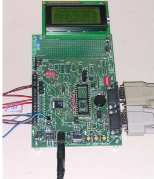
Figure 7.4.1: MSC1211 evaluation board.
