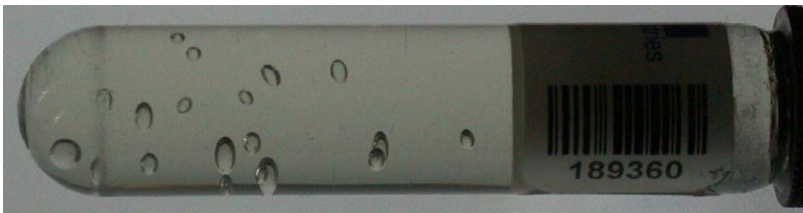
Figure 7: Digital photograph of a bubble detector irradiated with neutrons in FLASH tunnel.
