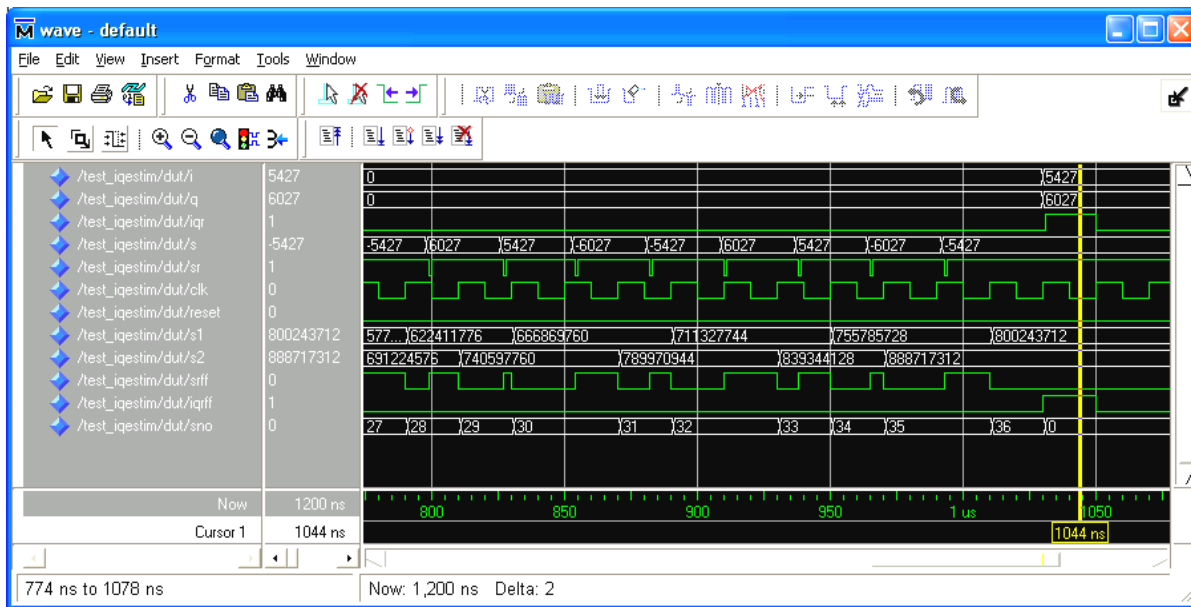
Fig. 4. IQ estimator ( IQestim VHDL module) - simulation results IF=81\text{MHz} , SF=36\text{MHz} time for sample collection -1\mu\text{s} therefore 36 samples taken into account output: I=5427 , Q=6027 , \Rightarrow A=8110 , \varphi=48^\circ
