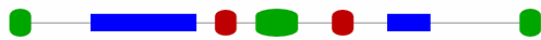
Figure 2: Forward cell of the dogleg. The cell length is about 2.53m as measured along curved beam path. Blue, green and red colours mark dipole, quadrupole and sextupole magnets, respectively.
