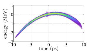
Figure 2: Longitudinal phase-space distribution measured after the seeding setup for an uncompressed electron bunch. The laser-induced energy modulation emerges as a region with larger slice energy spread.
