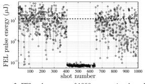
Figure 3: FEL pulse energy of 1000 consecutive shots. Between shot number 400 and 650, the seed laser shutter was closed.
