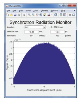
Figure 7: Beam energy spectra measured with the synchrotron radiation cameras in the chicanes are plotted for the chicanes as a tuning aid.
