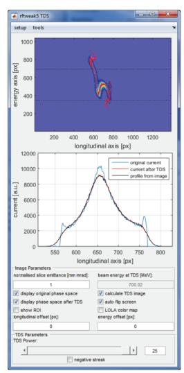
Figure 5: A simulated view of the LOLA transverse deflecting structure image for FLASH. The longitudinal phase space (red) is compared with the estimated image on the corresponding screen.
