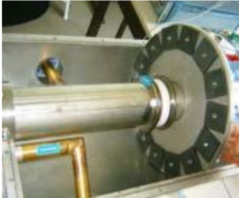
Figure 2: Inside view of the kicker cavity – direct look at the ferrite loaded moveable wall.
