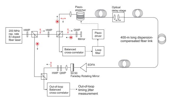
Figure 2: Experimental setup for the fiberlink stabilization.
