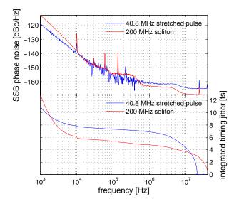
Figure 1: Phase noise comparision between a  $40.8\,\mathrm{MHz}$  stretched-pulse laser and a  $200\,\mathrm{MHz}$  soliton laser. Top: single-sideband phase noise measured at the harmonics at 980 MHz (stretched-pulse) and 1.2 GHz (soliton), respectively. Bottom: integrated timing jitter starting integration at  $20.4\,\mathrm{MHz}$  (stretched-pulse) and  $40\,\mathrm{MHz}$  (soliton). The measurements for the stretched-pulse laser are from [2].
