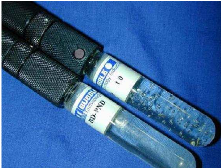
Figure 4: Picture of a bubble dosimeter; the upper one is irradiated and bubbles have formed.
