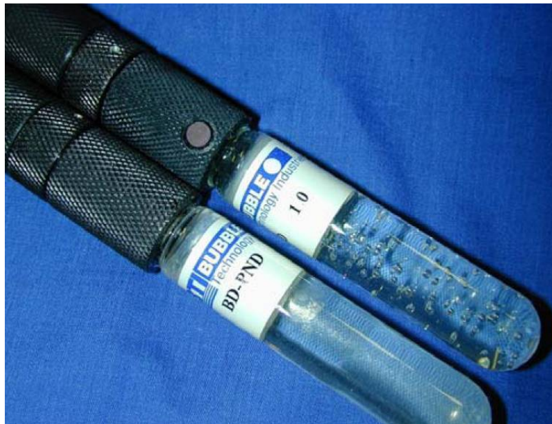
Figure 2.5: Neutron bubble detector [24].
