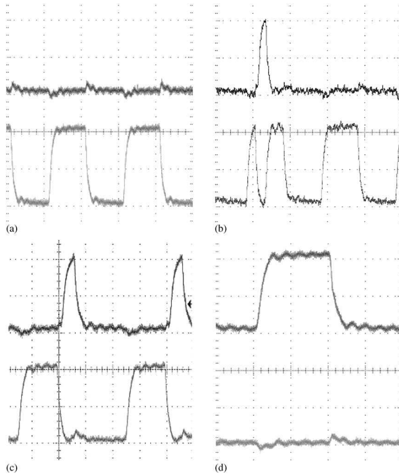
Fig. 3. Performance of the shift register design observed on the scope. Upper signal—the output of the XOR gate, bottom signal—the output of the shift register: (a) normal operation, (b) expected dynamic SEU signal, (c) the shift register is broken off, the functionality of the design is changed, (d) the shift register is broken off, input of the remained rearmost part of the register is connected to '0'.
