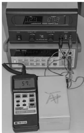
Figure 5. LEDs test system, consisting of light meter (RS V10860), multimeter (HP 34401A) and power supply (EA-PS 2016-050).
