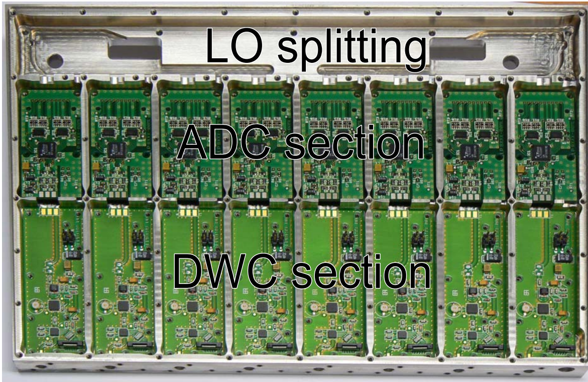
Figure 4.8: DWC prototype boards and ADC boards in the metal housing.
